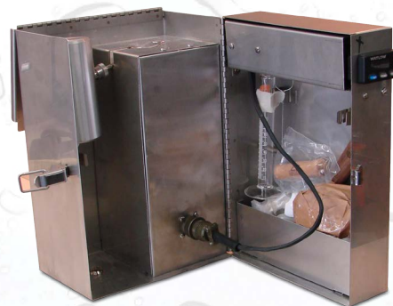
20 mL Retort Kit with Electronic Temperature Control
