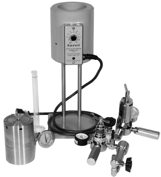
HPHT Filter Press, Model 175CT, CO 2 Pressurized Maximum Pressure: 1800 psig Backpressure: 750 psig Maximum Temperature: 350° F
