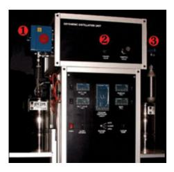
The Cryogenic Distillation System is used to isolate a gas fraction and liquid fraction from a lean, single-phase hydrocarbon system. From the measured masses of two fractions and the compositional analysis of each fraction, the original single-phase fluid composition can be calculated.
