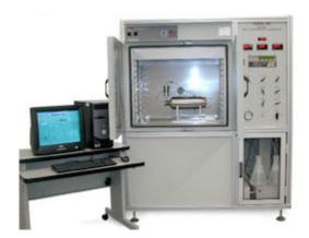
The Rock Compressibility RCA-841 measures the changes in pore volume and bulk volume as a function of axial, radial, and pore pressures. Effective stress and simulated reservoir stress can be measured. The system uses Core Lab's patented Tri-Axial Type Core Holder for independent application of axial, radial and pore pressure.
